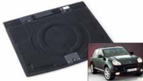
The rear cargo area load floor of the Porsche *Cayenne* is composed of structural layers of natural fiber composites surrounding an expanded polypropylene foam core and covered with a carpet cloth. All materials are comolded in a single, low-pressure press cycle. The floors are also used on the Volkswagen *Touareg* and new Audi Q7 vehicles, built on the same platform. Source: Quadrant Natural Fiber Composites
