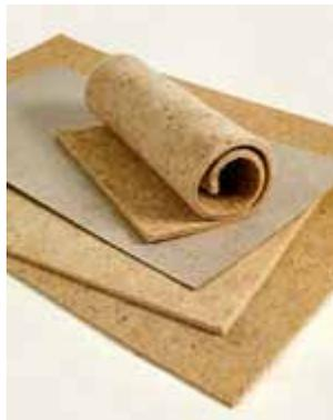
Different forms of natural fiber composite mats offered by FlexForm Technologies. The selection of mat (shown twice), LD (low-density), or HD (high-density) material is dependent upon the various heating methods used. All are 50 percent natural fiber and 50 percent synthetic fiber. Source: Flexform Technologies
