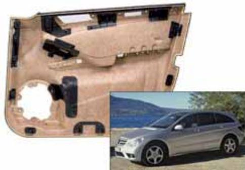
A door panel from the new Mercedes M-Class and R-Class (inset) platforms highlights the moldability characteristics of natural fiber. The back side attachments (dark color) are preloaded into the tool and bonded to the natural fiber composite during molding without resort to adhesives, a key factor in labor and material savings. Source: Flexform Technologies
