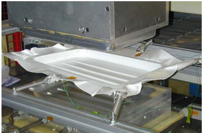
Thermoforming of suitcase shell from PURE® self-reinforced polypropylene sheet.
