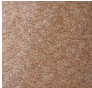
Gornaf® natural fiber reinforced thermoplastic sheet.
