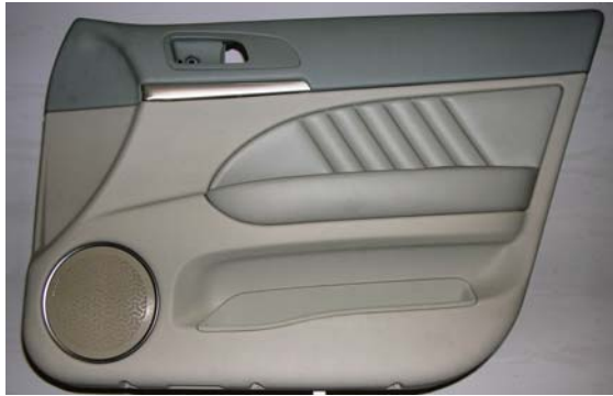
A door panel for the Alfa Romeo 159 sportwagon made by Johnson Control using Wood-Stock® thermoformable sheet material.
