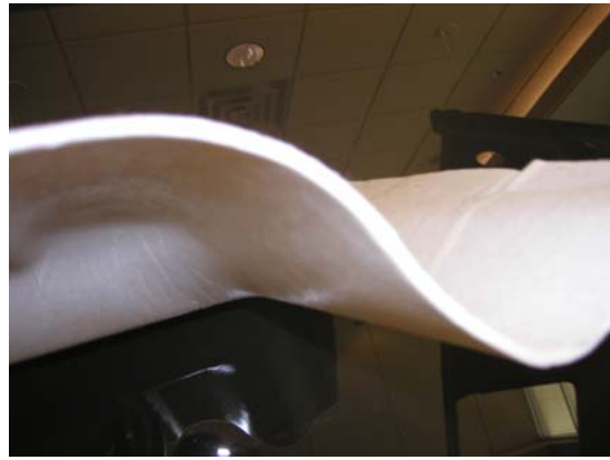
Side view of a molded headliner using AcoustiMax® fiber-reinforced thermoplastic, showing typical thickness.
