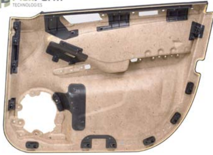
Automotive door liner made with FlexForm® composite sheet shows how fasteners can be bonded and integrated during a one-shot thermoforming process.
