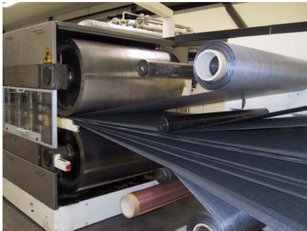
PURE® all-PP sheets are made by compacting multiple layers of highly oriented polypropylene tapes into a single consolidated composite.
