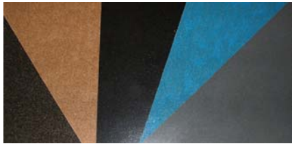
Wood-Stock® wood flour reinforced polypropylene composite sheets are used in automotive applications.
