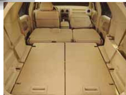
FlexForm's natural fiber composite is used on the backside of the second row, three-person bench in the Ford Freestyle SEL.
